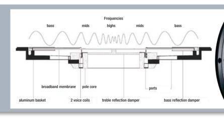
The thin, flexible membrane is completely flat.
