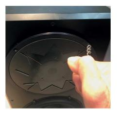
Place the removal tool or corkscrew in the screw hole opposite the remaining screw and tilt it slightly. You must now pull slowly and evenly so that the sealing tape behind the sound transducer slowly comes away from the housing. This can take some time.
