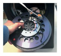
If the chassis has come loose, then remove the 4. screw. Rotate the MSW down to remove the cable ties and loosen clamps. At the terminals, like here in the picture you have to fold up the orange levers. Leave the terminals on the interior wiring.
