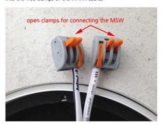
clean the interieur to avoid any damage on the MSW unpack the MSW carefully (Attention! Strong magnet!) connect the MSW
