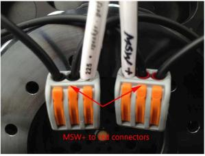
hold the MSW upside down, so that the MSW connectors can be clamped - see photo
