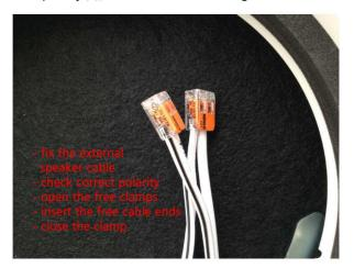
clamped the stripped ends of the external speaker cable into the free clamps of the IN+/IN cables
