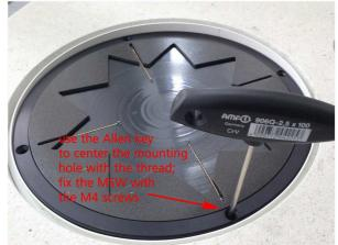
place the MSW in the cabinet, adjust the MSW with the Allen key; don't fix the MSW to strong as the damping rings are soft and will be compressed
