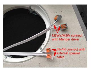
internal connectors comes with clamps lift the orange lever for open the clamps
