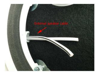
push the external speaker cable cable length pulled through should be around 200 - 300 mm (8 - 12")
