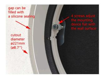
adjust the mounting ring so that is flat with the wall surface
