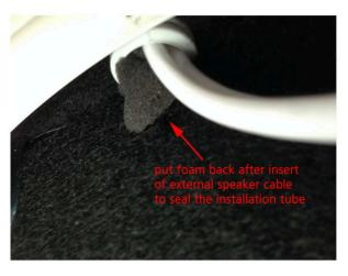
push foam into the installation tube to seal it
