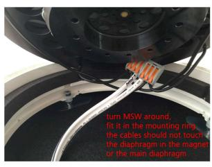
turn the MSW around - push the internal cable below the mounting ring - check that the holes are at the right position
